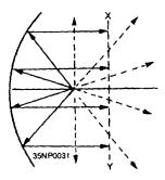
Figure 2-39.—Parabolic reflector radiation.
