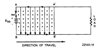
Figure 3-7.—Dc voltage applied to a line.
