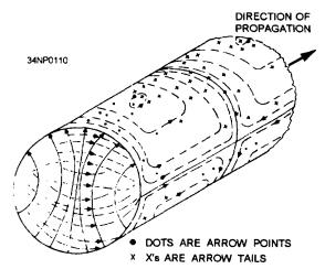
Figure 3-37.—Dominant mode in a circular waveguide.
