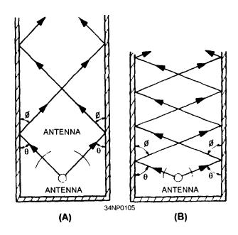
Figure 3-32.—Different frequencies in a waveguide.
