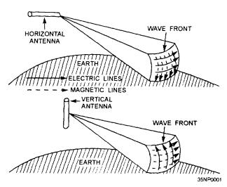
Figure 2-2.—Horizontal and vertical polarization.
