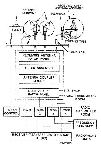
Figure 2-38.—Receive signal distribution system.
