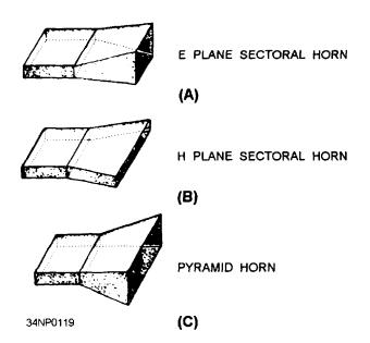
Figure 3-46.—Waveguide horns.
