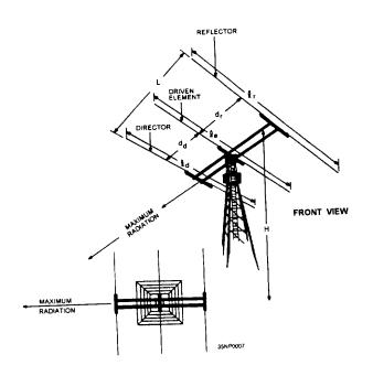
Figure 2-15.—Yagi antenna.
