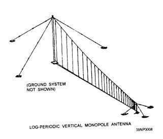
$\label{periodic vertical monopole} \textbf{Figure 2-16.--Log-periodic vertical monopole} \\ \textbf{antenna.}$
