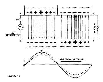
Figure 3-8.—Ac voltage applied to a line.
