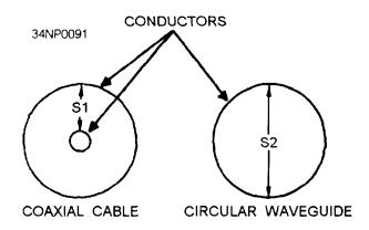
Figure 3-18.—Comparison of spacing in coaxial cable and a circular waveguide.
