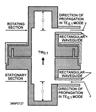
Figure 3-54.—Rotating joint.
