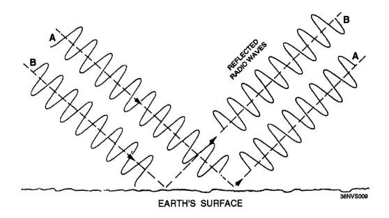
Figure 1-9.—Phase shift of reflected radio waves.
