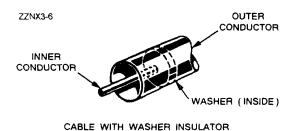
Figure 3-13.—Air coaxial line.
