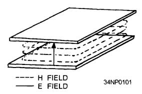
Figure 3-28.—H field boundary condition.
