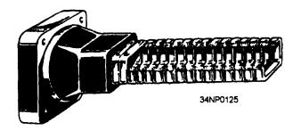
Figure 3-52.—Flexible waveguide.
