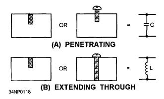
Figure 3-45.—Conducting posts and screws.
