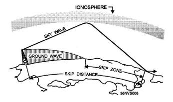
Figure 1-8.—Relationship between skip zone, skip distance, and ground wave.
