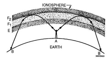
Figure 1-3.—Radio-wave refraction.
