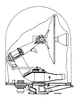
Figure 2-36.—Four-foot shf SATCOM antenna.
