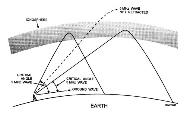
Figure 1-7.—Effect of frequency on the critical angle.
