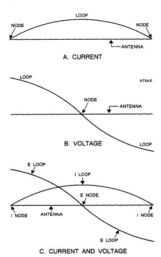
Figure 2-4.—Standing waves of current and voltage on an antenna.
