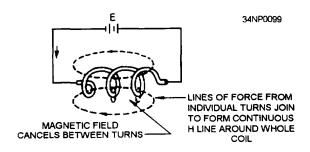
Figure 3-26.—Magnetic field on a coil.
