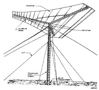
Figure 2-18.—Rotatable log-periodic antenna.
