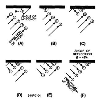
Figure 3-31.—Reflection of a single wavefront.
