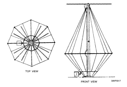
Figure 2-25.—AS-2802/SCR discage antenna.
