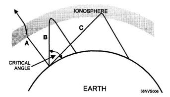
Figure 1-6.—Incidence angles of radio waves.
