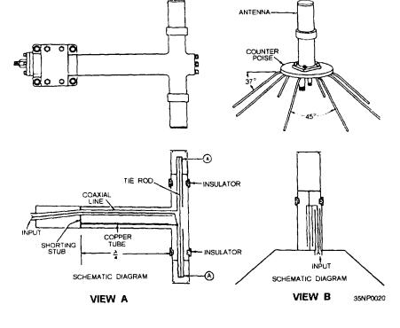
Figure 2-28.—Coaxial dipole.
