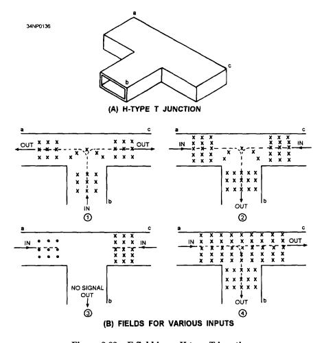
Figure 3-63.—E field in an H-type T junction.
