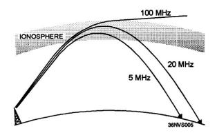
Figure 1-5.—Frequency versus refraction and distance.
