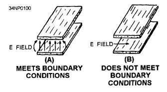
Figure 3-27.—E field boundary condition.
