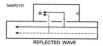
Figure 3-58.—Directional coupler designed to sample retlected energy.
