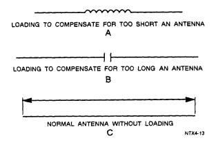
Figure 2-8.—Electrical antenna loading.
