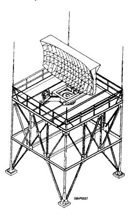
Figure 2-45.—AN/GPN-27(ASR-8) air surveillance radar.
