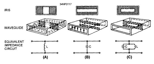
Figure 3-44.—Waveguide irises.
