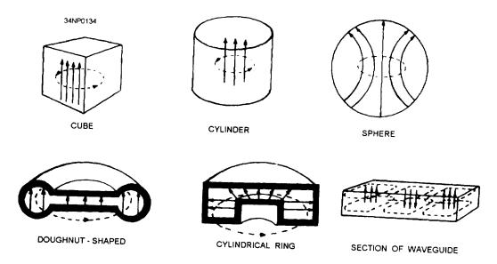
Figure 3-61.—Types of cavities.
