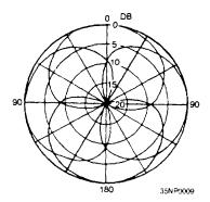
Figure 2-17.—Sector LPA and its horizontal radiation pattern.
