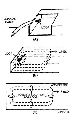
Figure 3-42.—Loop coupling in a rectangular waveguide.
