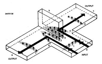
Figure 3-66.—Magic-T with input to arm d.
