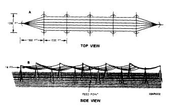
Figure 2-10.—Triatic-type antenna.
