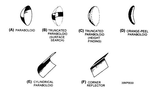
Figure 2-41.—Reflector shapes.
