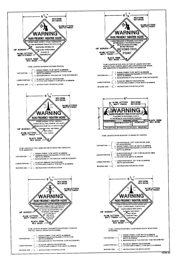
Figure 2-49.—Rf radiation warning signs
