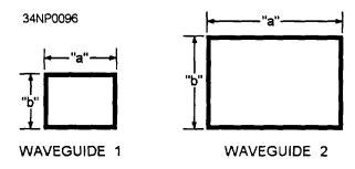
Figure 3-23.—Labeling waveguide dimensions,
