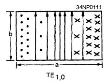
Figure 3-38.—Dominant mode in a rectangular waveguide.
