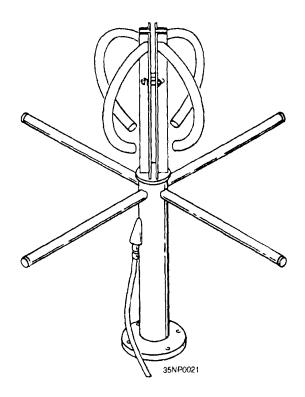
Figure 2-29.—AS-2815/SSR-1 fleet broadcast satellite receiving antenna.
