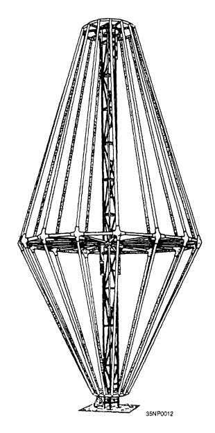
Figure 2-20.—Conical monopole antenna.
