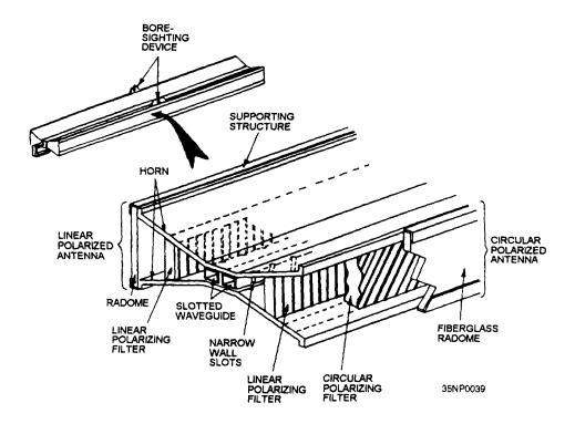
Figure 2-47.—SPS-55 antenna cross section.
