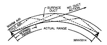
Figure 1-14.—Duct effect caused by temperature inversion.
