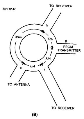
Figure 3-69.—Hybrid ring with wavelength measurements.
