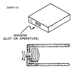
Figure 3-43.—Slot coupling in a waveguide.
