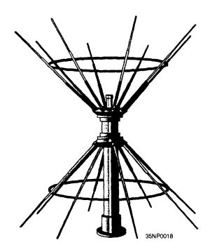
Figure 2-26.—AS-2811/SCR biconical dipole antenna.
