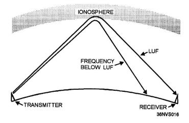
Figure 1-16.—Refraction of frequencies below the lowest usable frequency (luf).
