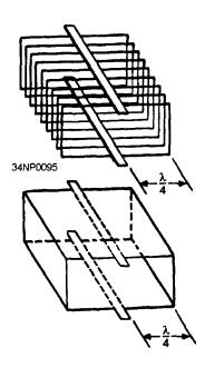
Figure 3-22.—Forming a waveguide by adding quarter-wave sections.
