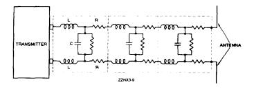
Figure 3-1.—Two-wire transmission line.
