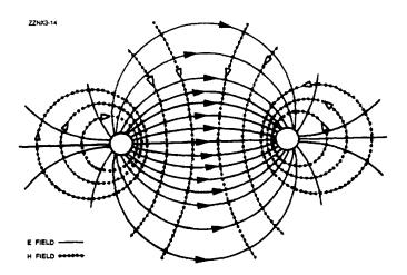
Figure 3-6.—Fields between conductors.
