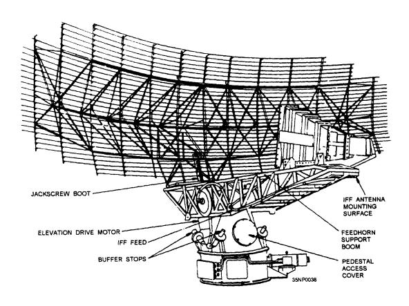
Figure 2-46.—AS-3263/SPS-49(V) antenna.
