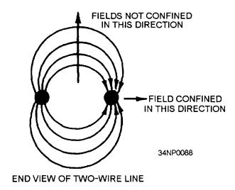
Figure 3-15.—Fields confined in two directions only.
