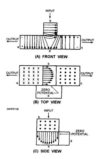
Figure 3-65.—Magic-T with input to arm b.
