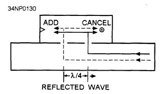
Figure 3-57.—Reflected wave in a directional coupler.
