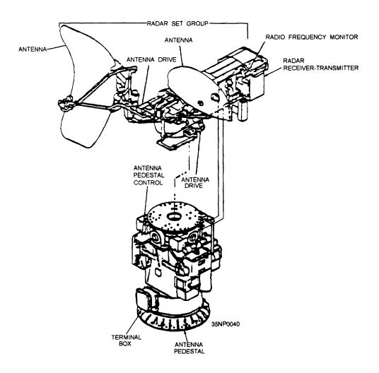
Figure 2-48.—AN/SPN-3SA aircraft control approach radar.
