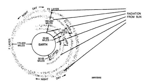
Figure 1-2.—Layers of the ionosphere.
