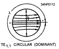
Figure 3-39.—Counting wavelengths in a circular waveguide.
