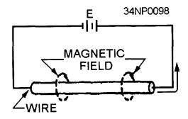
Figure 3-25.—Magnetic field on a single wire.
