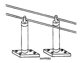
Figure 3-19.—Two-wire transmission line.
