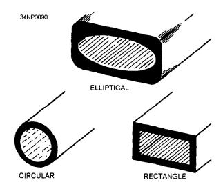
Figure 3-17.—Waveguide shapes.
