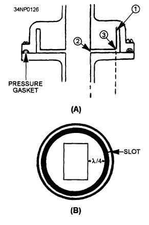
Figure 3-53.—Choke joint.
