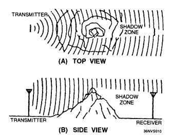
Figure 1-10.—Diffraction around an object.
