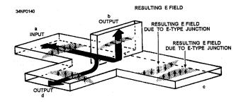
Figure 3-67.—Magic-T with input to arm a.
