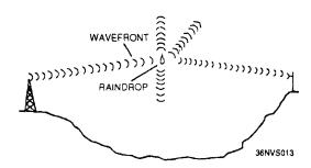
Figure 1-13.-Rf energy losses from scattering.
