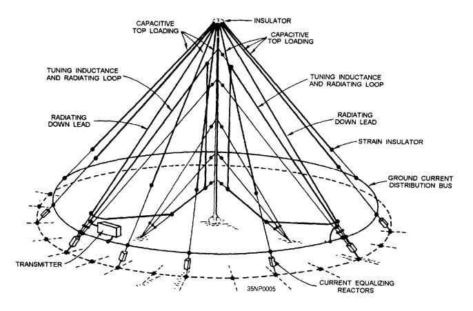
Figure 2-13.—Pan polar antenna.
