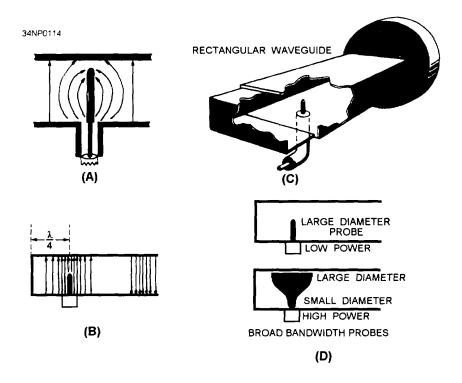
Figure 3-41.—Probe coupling in a rectangular waveguide.
