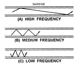
Figure 3-33.—Reflection angle at various frequencies.
