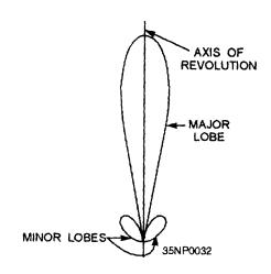
Figure 2-40.—Parabolic radiation pattern.
