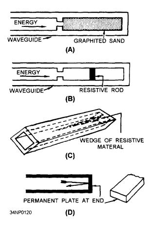
Figure 3-47.—Terminating waveguides.
